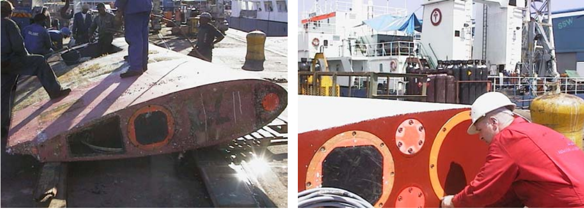
Figure 2 Transducer arrangement of the drop keel of R/V “Dr. Fridtjof Nansen” showing schematic illustration of the new orientation of the transducers on the keel (scale 1:10) (a) and photo taken before (b) and after (c) the refit in Cape Town in January 2001.
