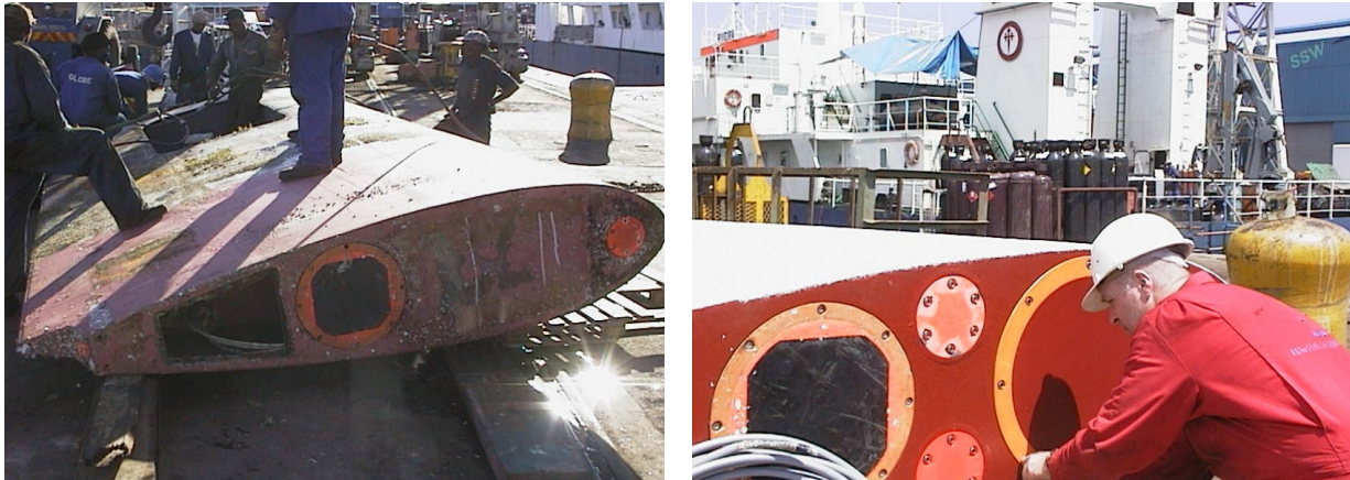
Figure 2 Transducer arrangement of the drop keel of R/V “Dr. Fridtjof Nansen” showing schematic illustration of the new orientation of the transducers on the keel (scale 1:10) (a) and photo taken before (b) and after (c) the refit in Cape Town in January 2001.
