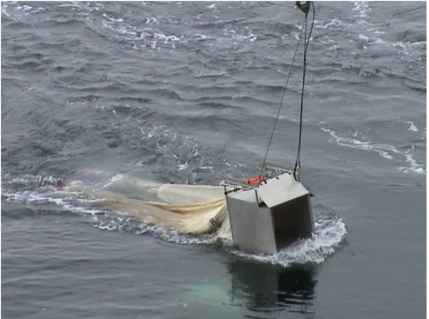
FIGURE 4. The Hydrobios multinet plankton sampler in the surface
