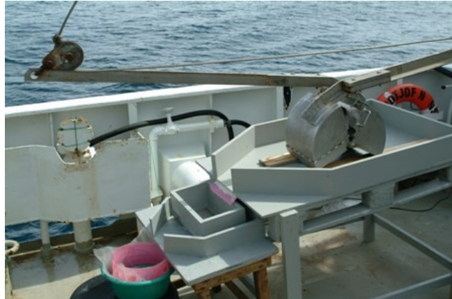
Figure 2. 0.1 m 2 Ven Veen grab and the arrangement of the table and sieves.
