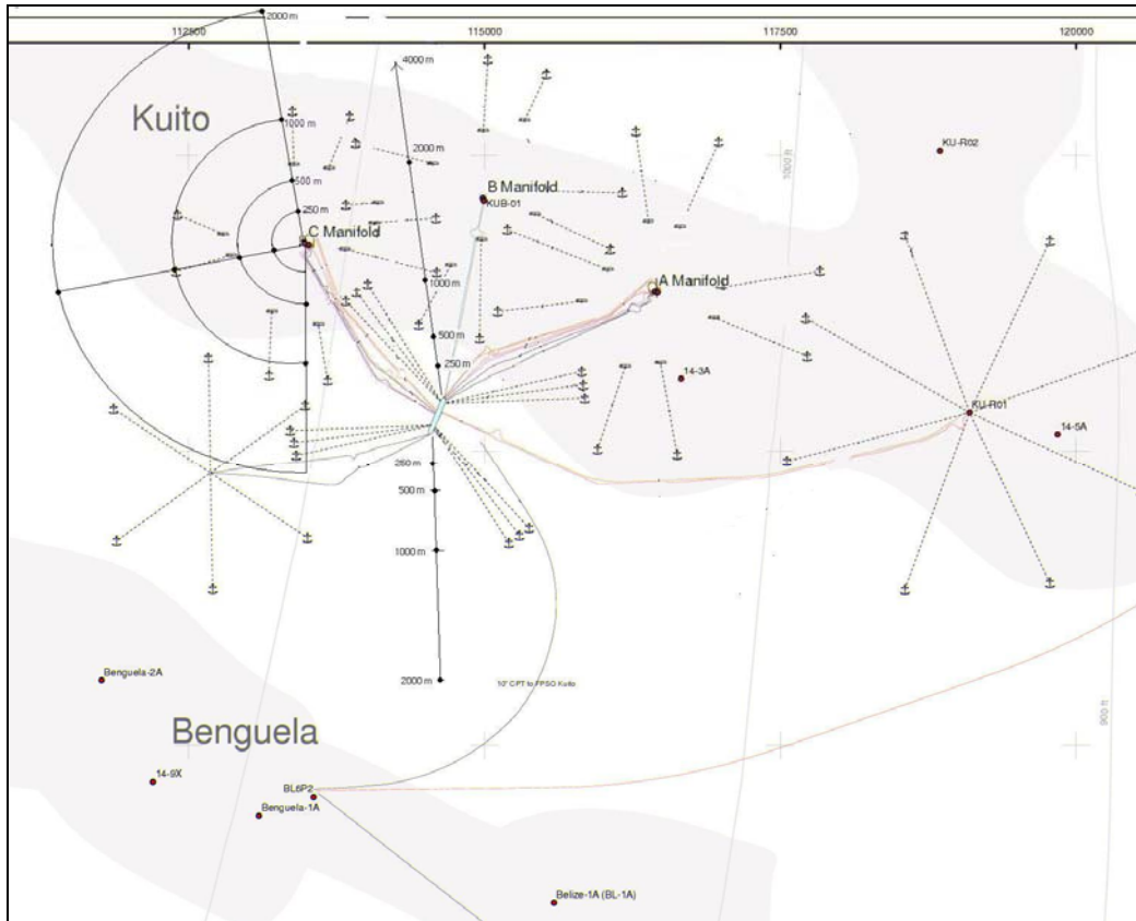
Figure 2.4 Detailed maps of the pipelines around Kuito (updated in 2006), and the proposed sampling design. The sites are located 250 m, 500 m, 1000 m and 2000 m north and south of FPSO. In addition one site 4000 m and 10000 m distance north of the FPSO will be taken. It is also planned to take samples along three transects from Manifold C (250 m, 500 m, 1000 m and 2000 m distance).
