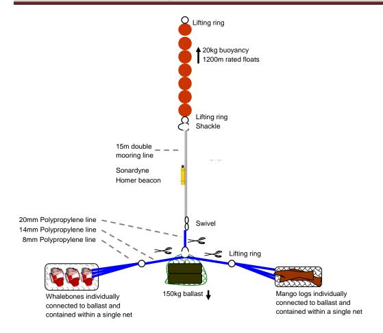
Figure 10.1 Mooring setup. The scissor symbol designates where the ROV should cut during recovery. See details later in the text.
