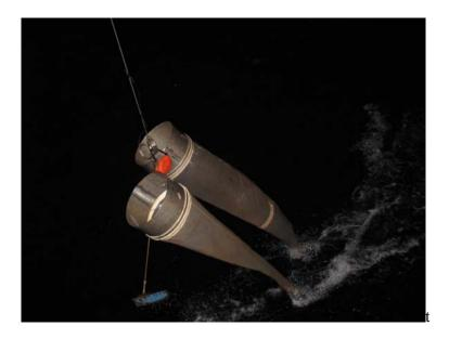
Figure 6.3 Night time deployment of Bongo nets with SCANMAR sensors (red) of the starboard side of the ship.
