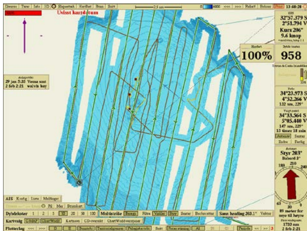
Figure 14a). Wüst seamount, Location 1 (western), showing surveys track and isobaths of the summit and adjacent slopes (10m depth contours). The shallowest central plateau is ca. 1050 m. Notice rugged knolls to the west of the central plateau.
