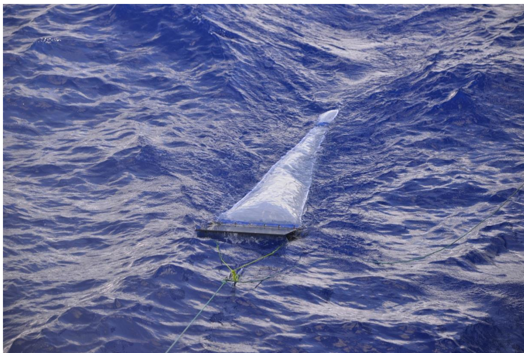
Figure 10, Manta Trawl sampling surface waters for microplastics and neuston communities. Note that the trawl used here does not have the flanking aquaplane panels typical of a manta design.
