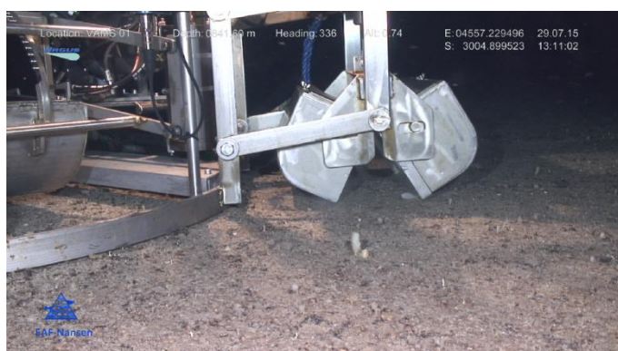
Figure 3.4.2. Image of the seabed observed at station MR. 08 (VAMS 01). The VAMS is attempting to close a grab on the hard substrate.
