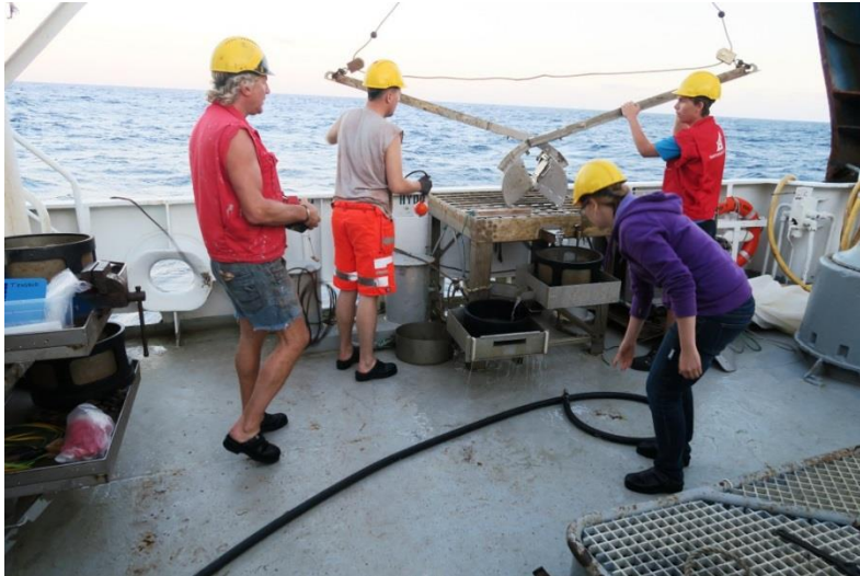
Picture 1.5.2 Sampling with the Van Veen grab.
