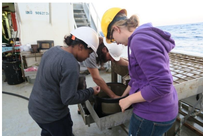
Picture 1.5.1 Asma, Javier and Lindsay sieving the sample from the Van Veen grab
