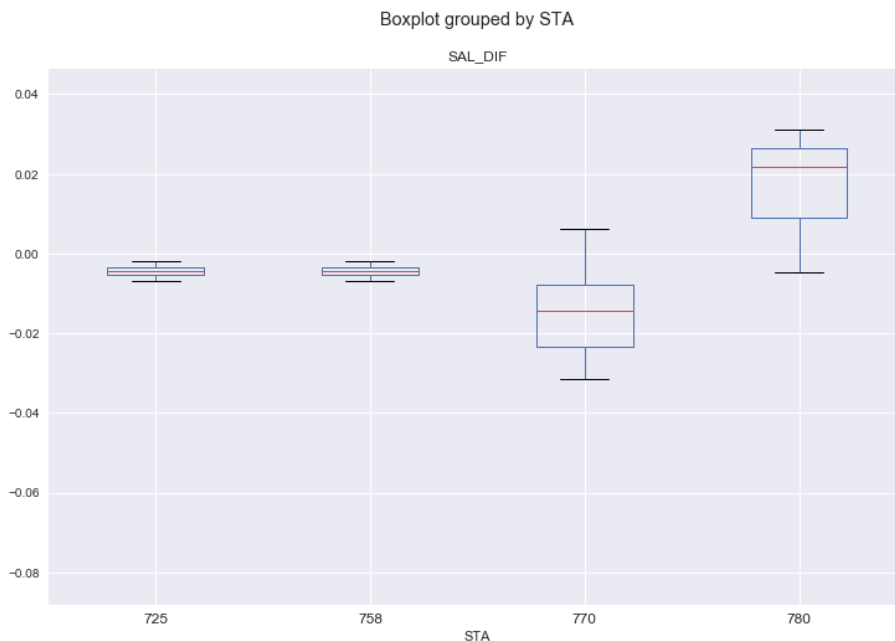
Figure VI.2. Median and quartiles of the difference between the salinometer and CTD-probe derived at the four stations sampled during survey 2017408. The horizontal axis describes station number, the vertical axis describes the difference between the salinometer and sensor derived variability.
