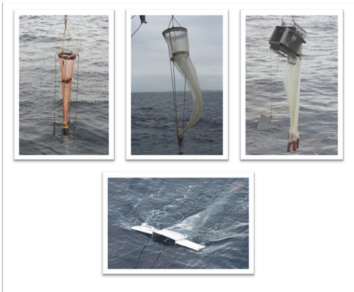
Figure 5. Plankton sampling equipment. Top: Phytoplankton net, WP2 net, Multinet rigged for oblique tow. Bottom: Manta trawl. Image credits: Jenny Huggett.
