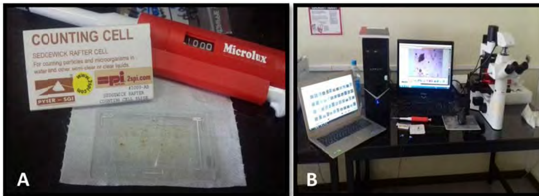
Figure A1.2: A. Loaded 1ml sample on Sedgewick rafter counting chamber; B. Analysis under a light microscope
