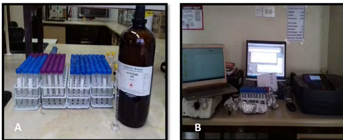
Figure A1.4: A. The addition of 10ml of 90% acetone, B. Analysis of sample using a spectrophotometer
