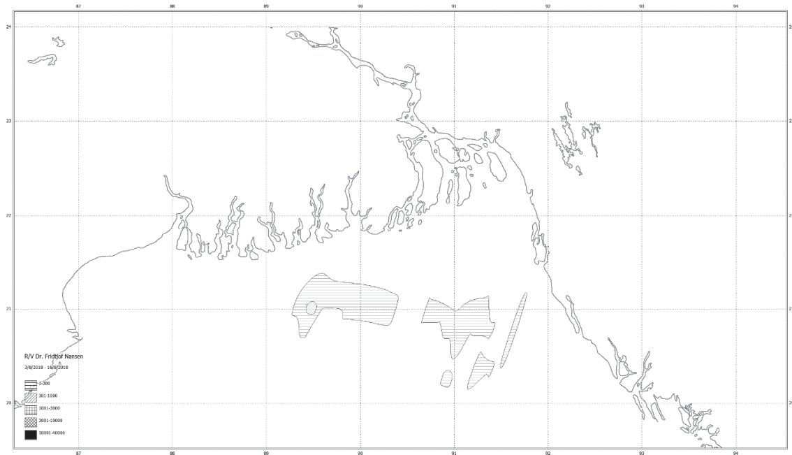
Figure 20. Acoustic backscatter strength of the PELAGIC 1 acoustic group determined from scrutinizing multi-frequency echograms using LSSS software and plotted in Nansis Maptool.
