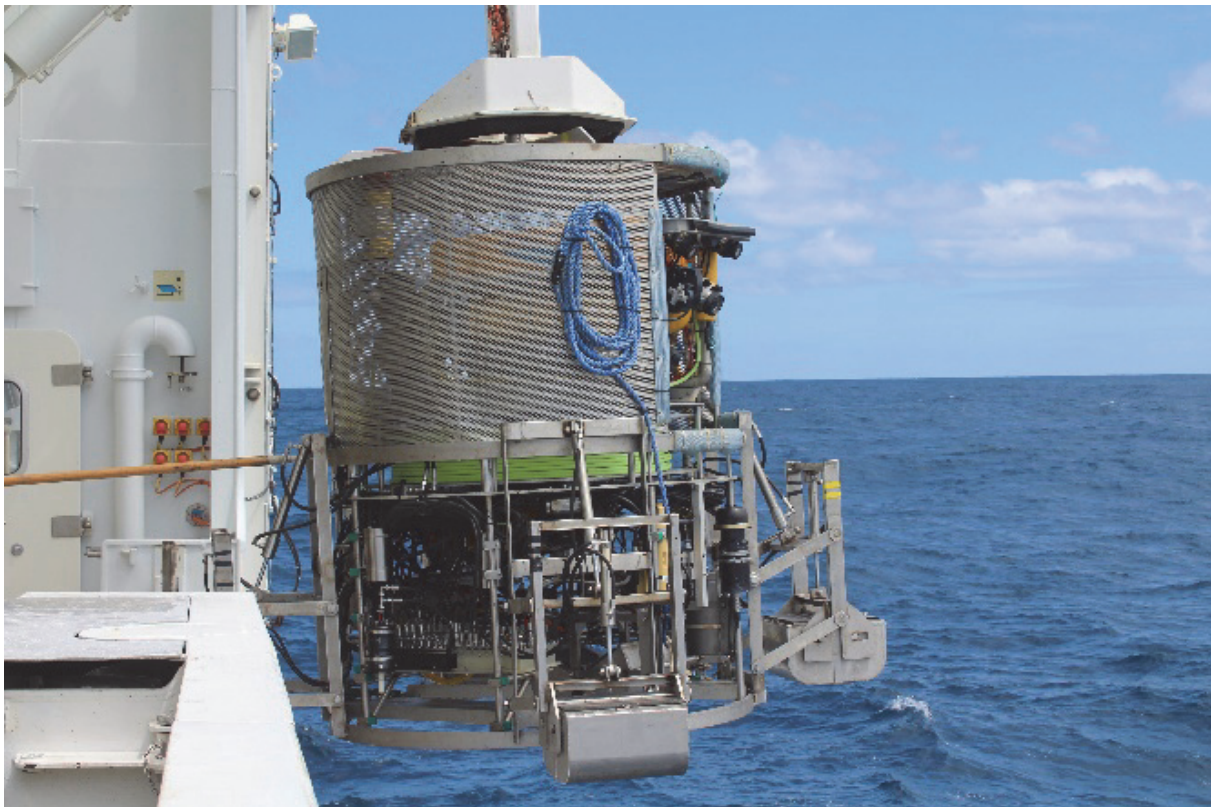
Figure 4. VAMS (Video-assisted Multi Sampler), used for observation and collection of benthos and habitats during the survey.
