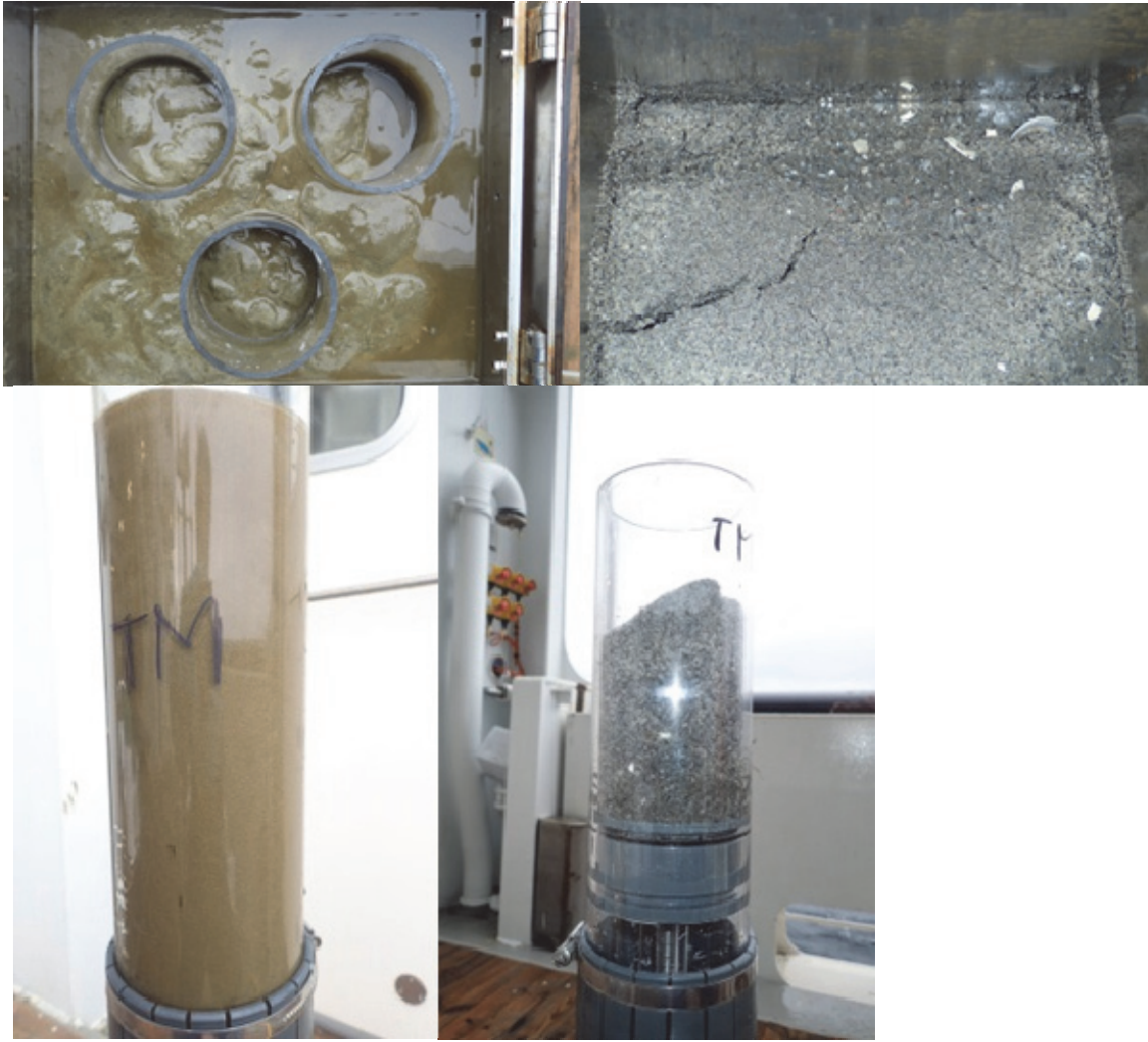
Figure 35. The surface of the two box cores and examples of the sub-cores that were collected
