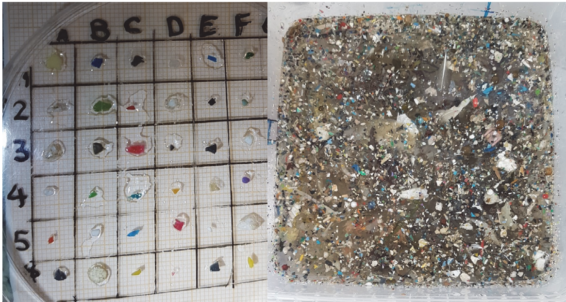
Figure 25. Microplastics found in the Manta net (left picture), and a sample with high concentration of microplastics (right picture)
