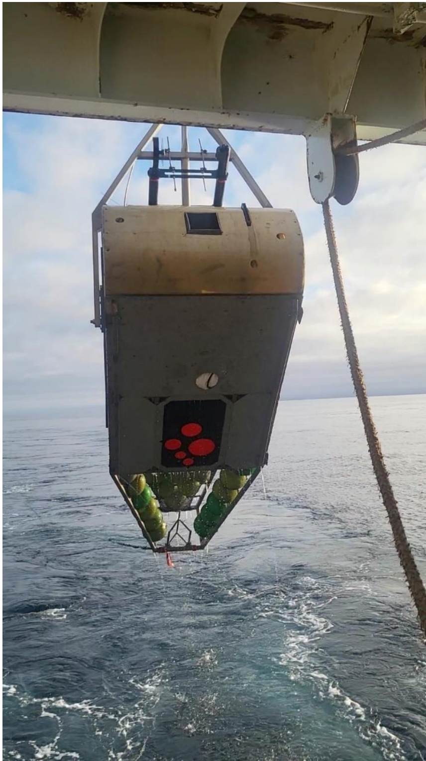
Figure 2: The towable echo sounder platform MESSOR developed for measurements in the mesopelagic zone. For the T2019001 dataset the position of the 333 kHz transduce was modified to be facing in a different angle, not shown in this picture. Photo: Kristian Rørhus Fjeld.
