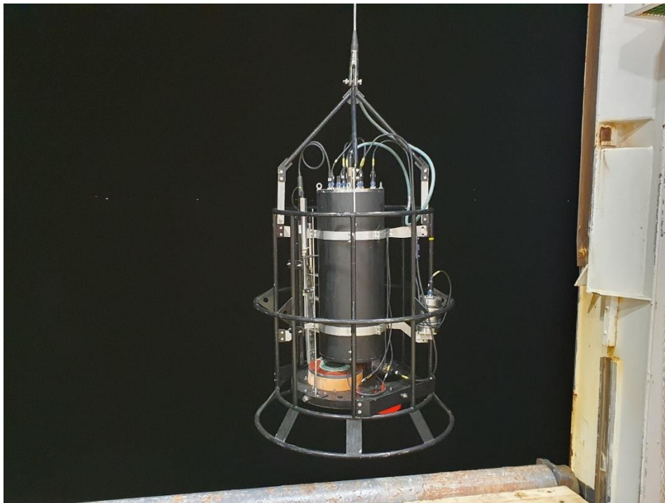
Figure 6: The TS probe with four transducers mounted to project downwards, held by crane on its way into the water. Photo: Rokas Kubilius
