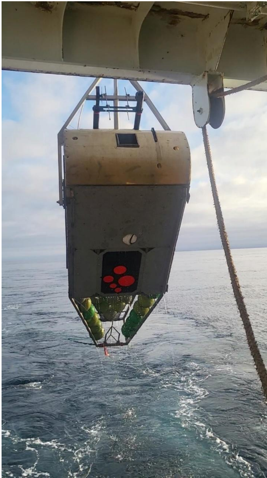
Figure 2: The towable echosounder platform MESSOR developed for measurements in the mesopelagic zone. For the T2019001 dataset the position of the 333 kHz transducer was modified to be facing in a different angle, not shown in this picture. Photo: Kristian Rørhus Fjeld.
