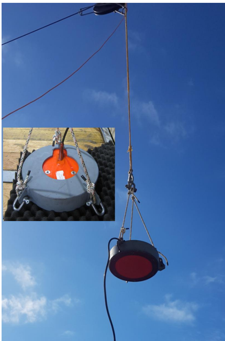
Figure 8: The submersible, narrow beamwidth (3 degrees) transducer (ES200-3C) mounted in a protective metal housing. The transducer was deployed by a rope over the side of the ship to 10 m depth, operated via 20 m transducer cable connected directly to a transceiver (Kongsberg EK80 WBT), which in turn was connected to a personal computer operating EK80 software. Photo: T.N. Forland/R. Kubilius
