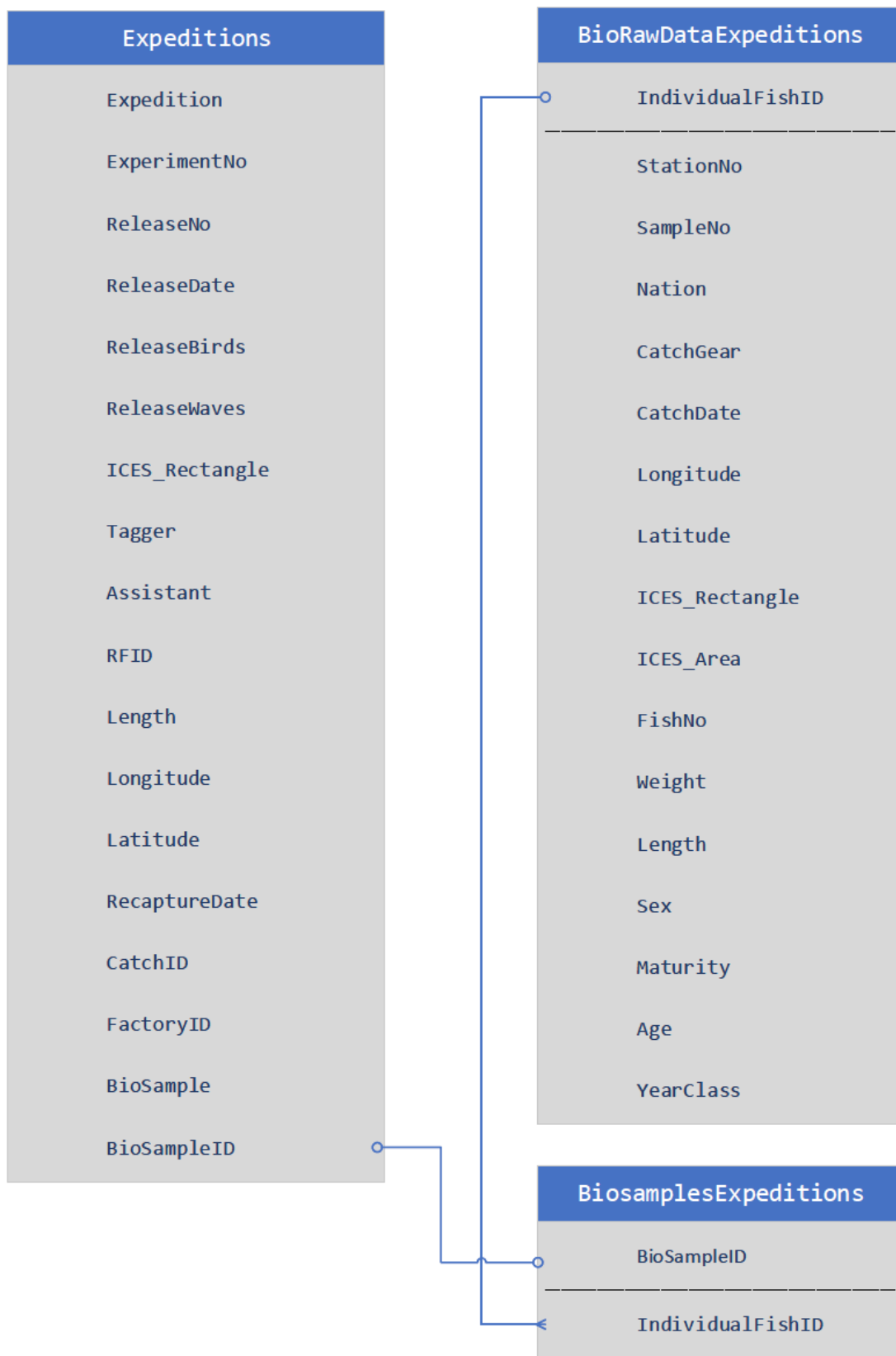
Figure 1. Overview of variables in the tagging expeditions and the links to exact biological data forming the basis for estimating numbers released and recaptured by age/year class as basis for stock assessment. Note that each tagged fish has an allocated BioSample, and based on Length at release and an ALK (Age Length Key) from individual Length and Age of fish in allocated BioSample, a relative age distribution is estimated for each tagged fish. This distribution follows from release until recapture. Hence, a single recapture would show probabilities (0-1) of ages based on release length, signifying that over a year the sum of recaptures per age will be with decimals. See Tables 1-2 for detailed explanations of variables.
