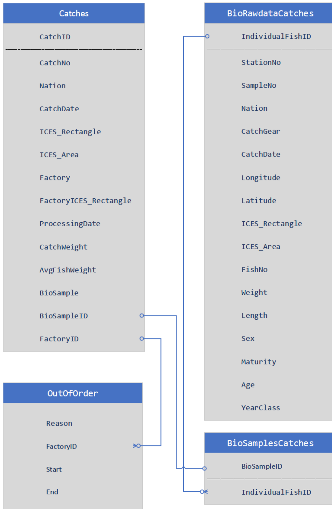
Figure 2. Overview of variables in the catch data and the links to exact biological data and info on factories/periods with unacceptable recapture efficiencies (OutOfOrder=not used in stock assessment) forming the basis for estimating numbers scanned by age/year class as input to stock assessment. Note that each catch has an allocated BioSample, and based on the relative age distribution of individual fish in this sample as well as number of fish in catch (CatchWeight/AvgFishWeight), numbers by age/year class can be estimated in same way as in the stock assessment. Note that AvgFishWeight is analysed per catch at each factory, but may occasionally be missed, and then AvgFishWeight should be same as average weight in the allocated BioSample.
