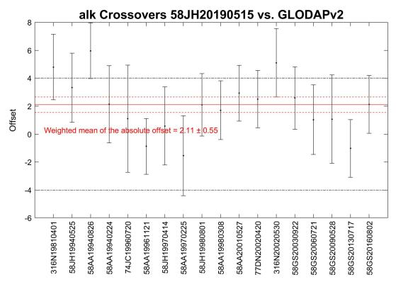
The lab-based analyzes are always 10-15 mmol kg<sup>-1</sup> higher than the ship-based analyzes where we have both. The reason is suspected to be evaporation prior to analysis in the lab. Measurements of DIC and pH were done on the same bottle before the AT analysis, and all analyzes were made during the warmest period of summer 2019 when temperatures in Bergen were close to or above  $30^{\circ}$ C. The lab is not air-conditioned.
