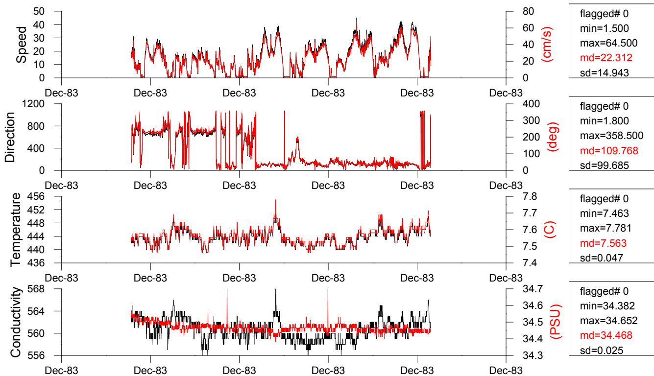
Note. Each graph contains time series in engineering (left axis, black curve) and physical (right axis, red curve) units.
