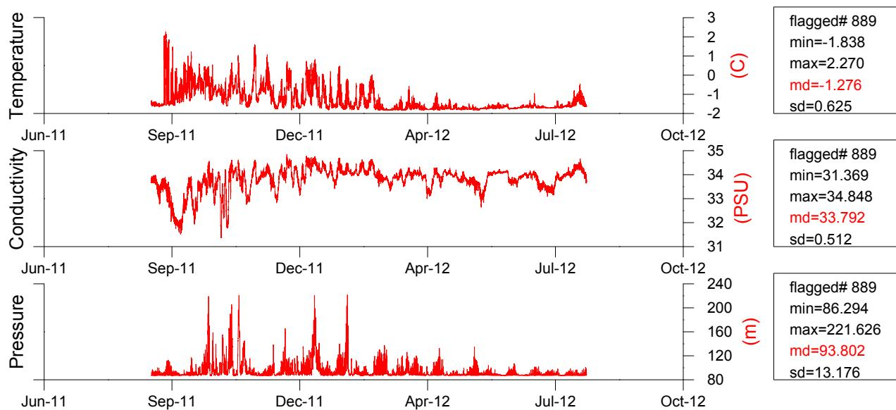
Note. Each graph contains time series in engineering (left axis, black curve) and physical (right axis, red curve) units.
