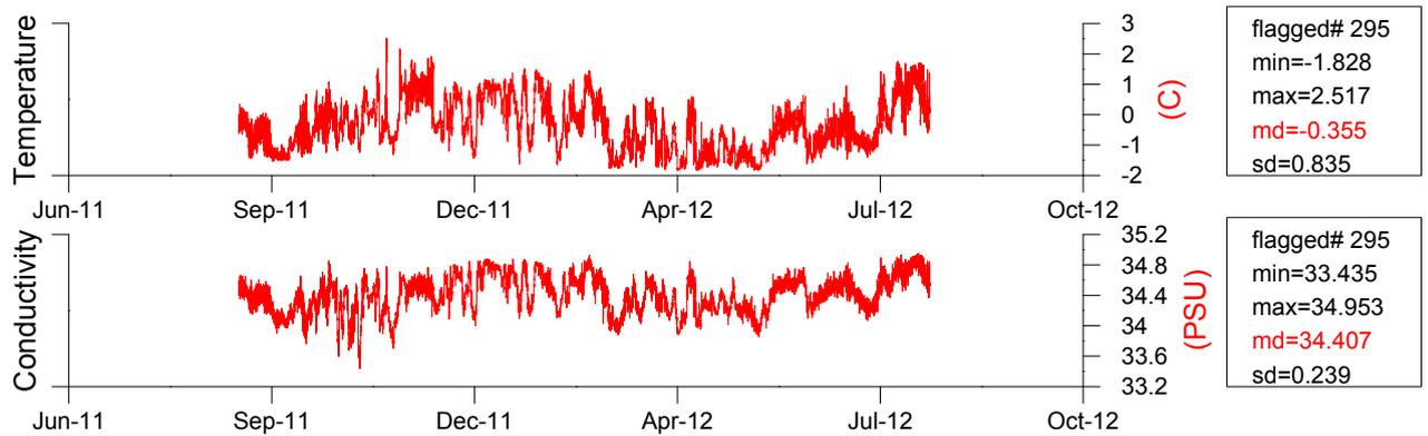
Note. Each graph contains time series in engineering (left axis, black curve) and physical (right axis, red curve) units. Number of flagged values as well min, max, mean and standard deviations in physical units are shown to the right.
