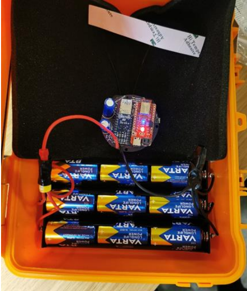
Figure 38: Battery pack designed for Uib01 as a drifter.
