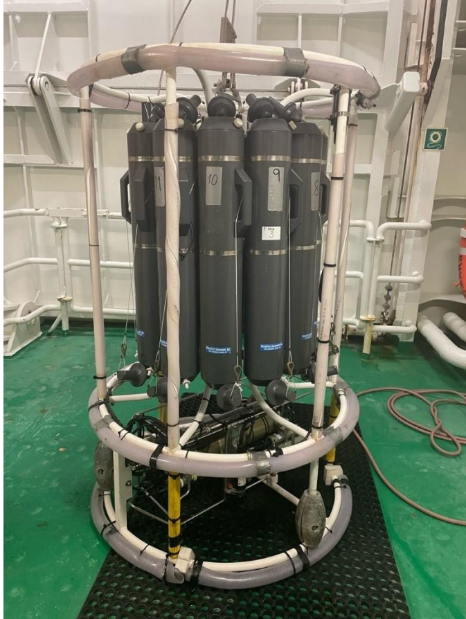
Figure 4: Picture of the CTD (Sea-bird 9 plus) used at G.O Sars. Photo: Astrid Berg Rosland, 2023
