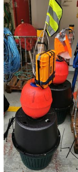
Figure 39: Uib01 ready to be deployed as a drifter.
