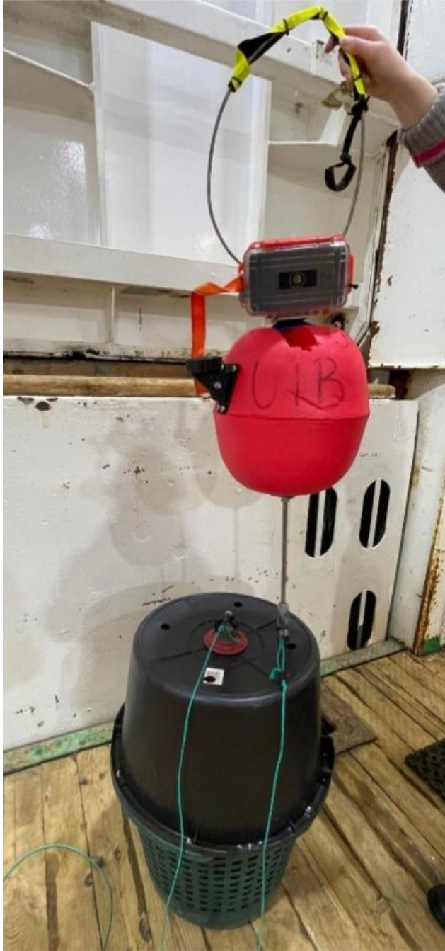
Figure 3: The image shows one of the drifters used during the cruise. From above: An orange box containing a lithium battery connected to a pole. The battery serves as a GPS tracker of the drifter's movements. Further down you will see a mooring buoy, which keeps the drifter afloat. Down below there is a thin, turquoise, 10-meter rope that is connected to two buckets. Inside the connected buckets there is a heavy chain. Photo: Nora Bringaker, 2023.
