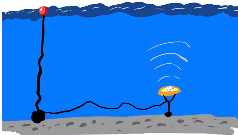
Figure 31: Illustrating the ADCP mooring setup at Haugsværffjorden. The red buoy is used for recovering the ECO-0342 ADCP.
