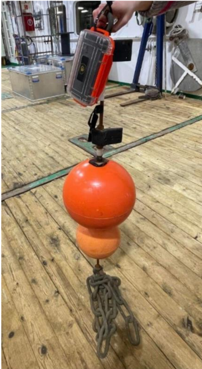
Figure 2: The image shows one of the drifters used during the cruise. From above: An orange box containing a lithium battery connected to a pole. The battery serves as a GPS tracker of the drifter's movements. Further down you will see two mooring buoys, which keeps the drifter afloat. Down below there is a heavy chain connected to the rod. Photo: Nora Bringaker, 2023.
