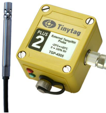
Figure 3.3.2: Picture of a TGP-4505 TinyTag, for measuring temperature and humidity.
