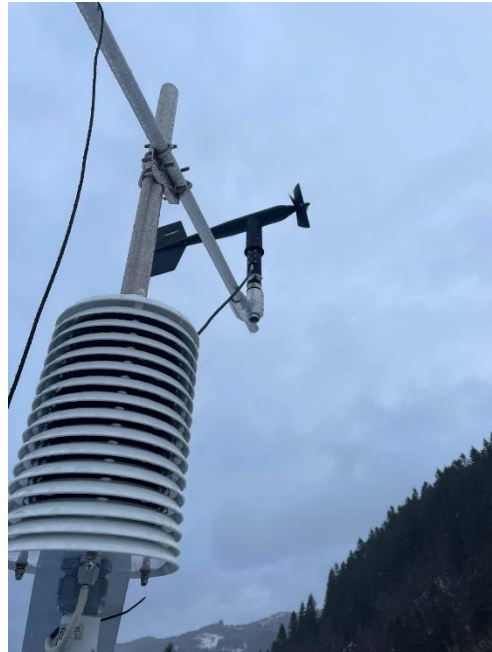
Figure 3.3.6: Picture of a R.M. Young 5106-45 Alpine wind speed- and wind direction sensor.
