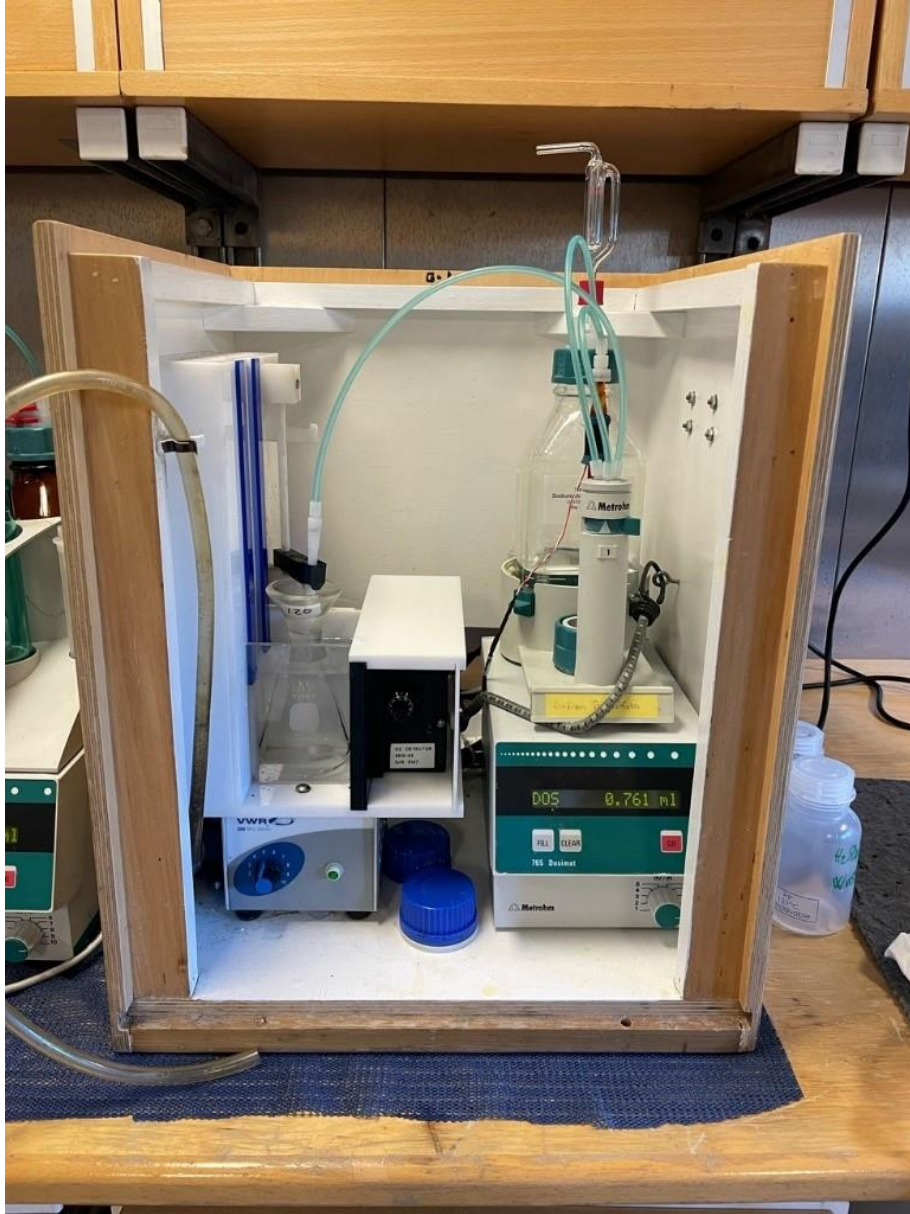
Figure 10: Semi-automatic titration device located in the laboratory on the G.O Sars.
