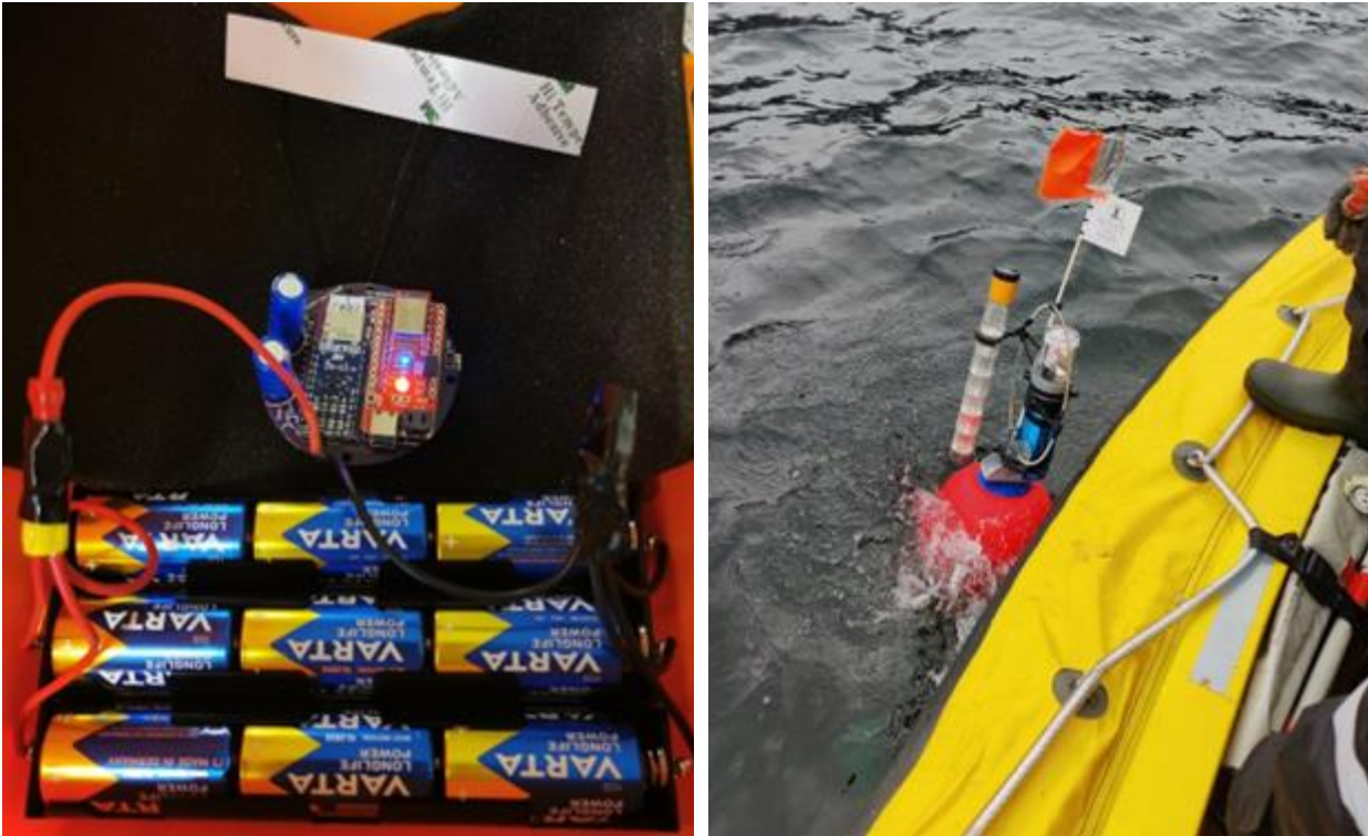
Figure 19: Overview of the wave measurement rig, to the left presenting the battery series connection and the microcontroller unit and to the right presenting the drifter in the water.
