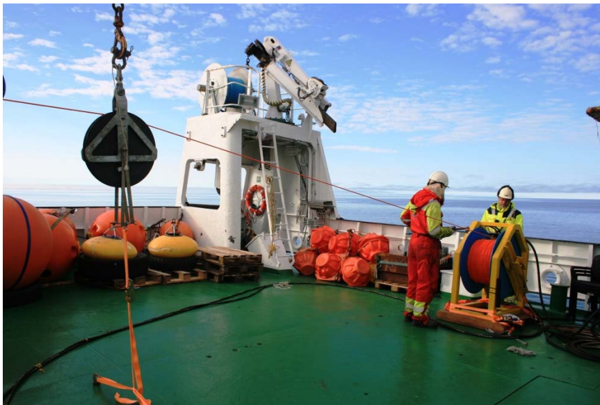
Figure 6. The set-up, on deck, of the VMP microstructure profiling system. The hydraulic winch (above); the cable is fed through a block supported by the crane in the middle. The block is fastened by straps to the deck to avoid swings due to wind and ship's roll. The tether then is fed into the line-puller (right) fastened to the ships' railing. In addition to the winch operator, a second person observes the cable in water during the deployment, and assists with deployment and recovery.
