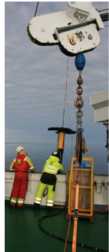
Figure 6. The set-up, on deck, of the VMP microstructure profiling system. The hydraulic winch (above); the cable is fed through a block supported by the crane in the middle. The block is fastened by straps to the deck to avoid swings due to wind and ship's roll. The tether then is fed into the line-puller (right) fastened to the ships' railing. In addition to the winch operator, a second person observes the cable in water during the deployment, and assists with deployment and recovery.
