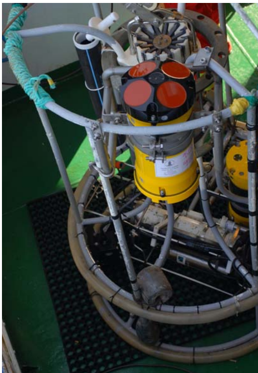
Figure 5. The CTD rosette together with the CTD sensors, one 10-liter Niskin bottle, a down and uplooker ADCP, and a benthos altimeter installed. The transducers of both ADCPs and the altimeter have a non-obstructed path. The position of the lead weights and the ADCPs are adjusted to have a negligible tilt of the entire system.
