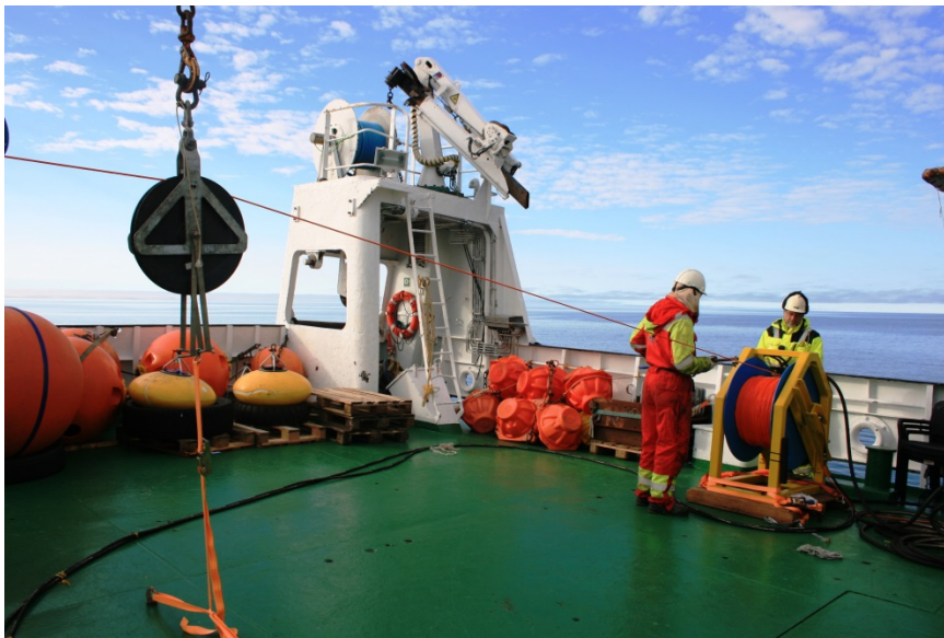
Figure 8. The set-up, on deck, of the VMP microstructure profiling system. The hydraulic winch (above); the cable is fed through a block supported by the crane in the middle. The block is fastened by straps to the deck to avoid swings due to wind and ship's roll. The tether then is fed into the line-puller (right) fastened to the ships' railing. In addition to the winch operator, a second person observes the cable in water during the deployment, and assists with deployment and recovery.
