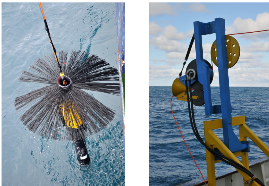
Figure 9. (Left) The VMP profiler during deployment. The brushes provide the drag for the profiler. Drag, together with the buoyancy elements (yellow) set the nominal sink velocity of the profiler. Note the recovery line attached to the cable which allows recovery by a crane without damaging the cable. (Right) The hydraulic line-puller.
