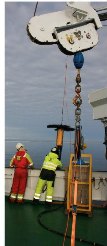
Figure 8. The set-up, on deck, of the VMP microstructure profiling system. The hydraulic winch (above); the cable is fed through a block supported by the crane in the middle. The block is fastened by straps to the deck to avoid swings due to wind and ship's roll. The tether then is fed into the line-puller (right) fastened to the ships' railing. In addition to the winch operator, a second person observes the cable in water during the deployment, and assists with deployment and recovery.
