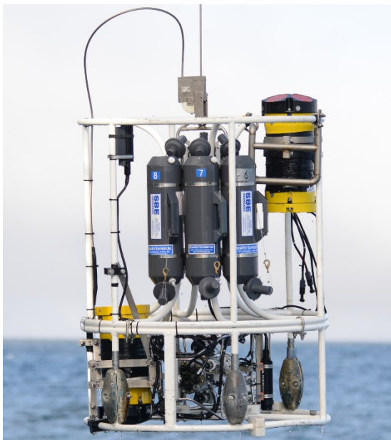
Figure 5. The CTD rosette together with the CTD sensors, three 10-liter Niskin bottles, a down and uplooker ADCP, and a benthos altimeter installed. The transducers of both ADCPs and the altimeter have a non-obstructed path. The position of the lead weights and the ADCPs are adjusted to have a negligible tilt of the entire system.
