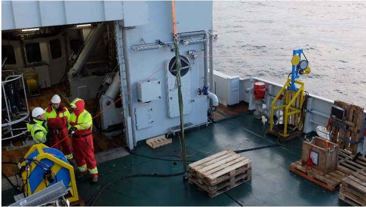
Figure 9. The set-up, on deck, of the VMP microstructure profiling system. The hydraulic winch (above); the cable is fed through a block strapped fixed at higher deck in the middle, and fastened by straps to the deck to avoid swings due to wind and ship's roll. The tether then is fed into the line-puller (right) fastened to the ships' railing. In addition to the winch operator, a second person observes the cable in water during the deployment, and assists with deployment and recovery.
