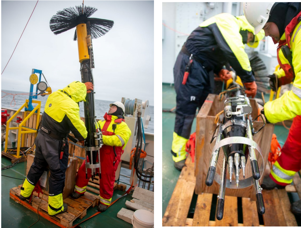
Figure 10. (Left) The VMP profiler during deployment. The brushes provide the drag for the profiler. Drag, together with the buoyancy elements (yellow) set the nominal sink velocity of the profiler. Note the recovery line attached to the cable which allows recovery by a crane without damaging the cable. (Right) The hydraulic line-puller.
