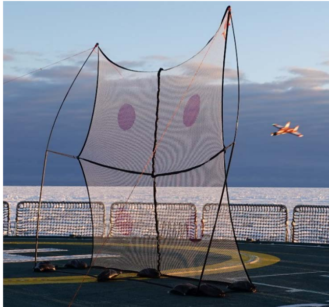
Figure 19. SUMO RPAS coming in for a net landing. The net is secured with sandbags and rope.
