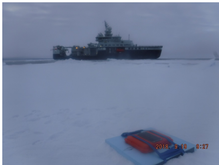
Figure 16. One of the wave in ice sensors deployed on a large ice floe. The main case containing the instrument, its solar panel, and the additional buoy around it are visible.
