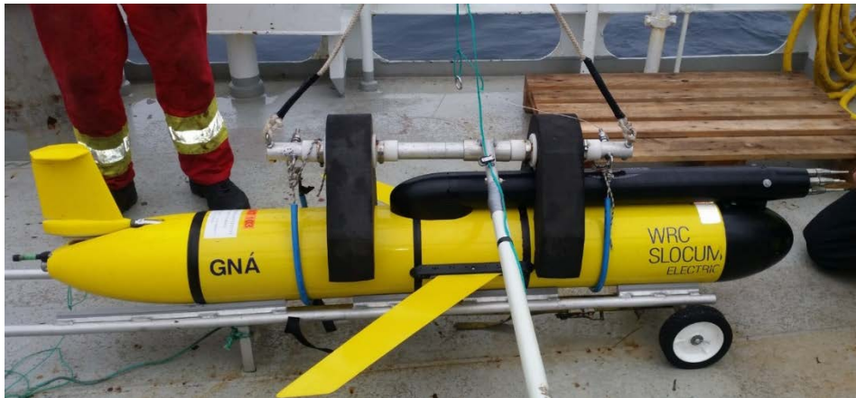
Figure 11. Photo of the glider Gná mounted with MicroRider, on the transportation trolley, together with the deployment tool.
