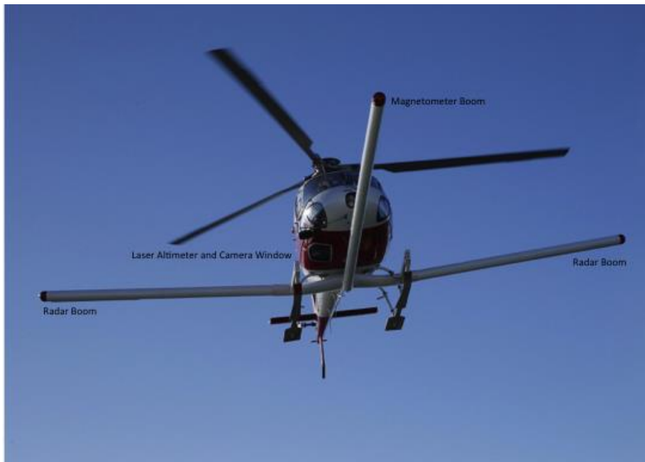
Figure 1.16. Configured survey helicopter with booms.
