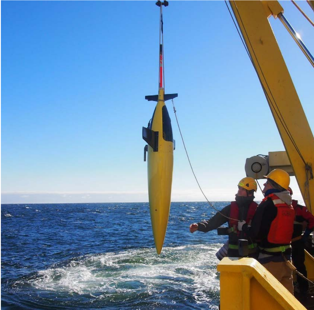
Figure 1.12. Seaglider being lowered to the water via slip stick lifting line looped around the rudder.
