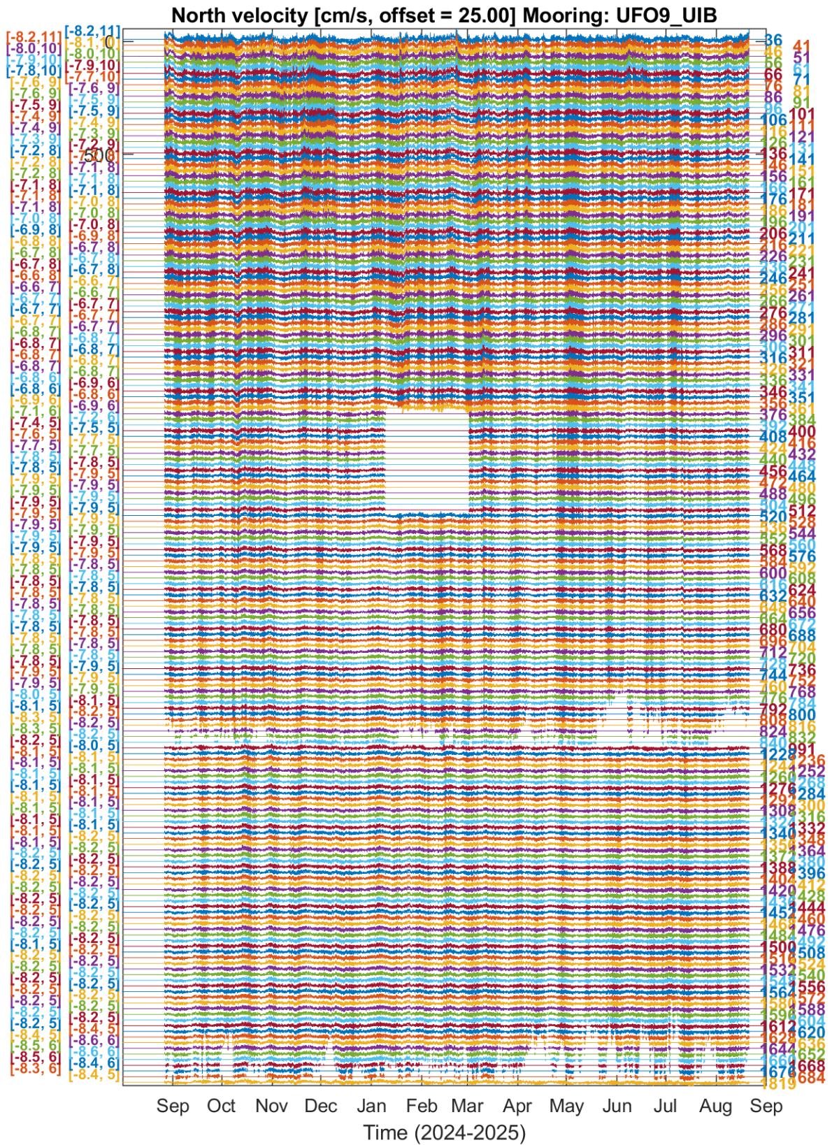
Figure 12. Time series of northward velocity. Numbers on the right (and the reference line) are the target depths. Numbers on the left show the time-averaged and 1 standard deviation values for the velocity records. The velocity records are shifted vertically by an offset of 25.00 cm/s for visualization purposes.
