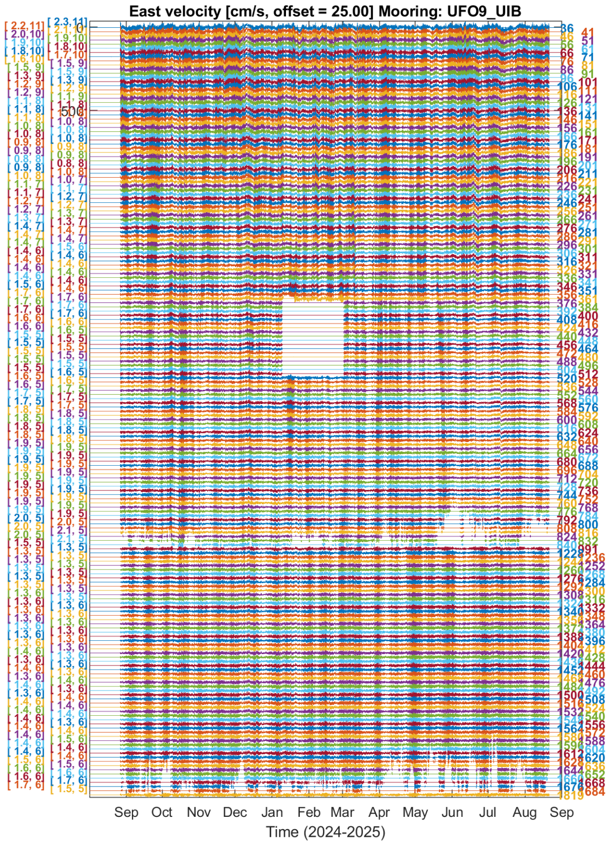
Figure 11. Time series of eastward velocity. Numbers on the right (and the reference line) are the target depths. Numbers on the left show the time-averaged and 1 standard deviation values for the velocity records. The velocity records are shifted vertically by an offset of 25.00 cm/s for visualization purposes.
