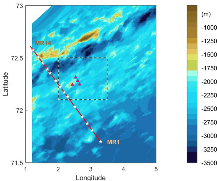
Figure 22. Multi-beam high resolution topography over the Mohn Ridge (data kindly provided by Rolf Birger Petersen, UIB). Red line with stations MR1 to MR14 mark the Mohn Ridge section. The dashed region is expanded in Figure 28. Triangles mark the seamount stations (Section 11.3).
