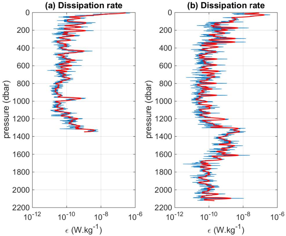
Figure 29. Dissipation profiles measured at (a) SM1 and (b) SM3 at the seamount site. Increased dissipation rates are clearly evidenced above and downstream of the seamount located below an horizontal frontal structure.
