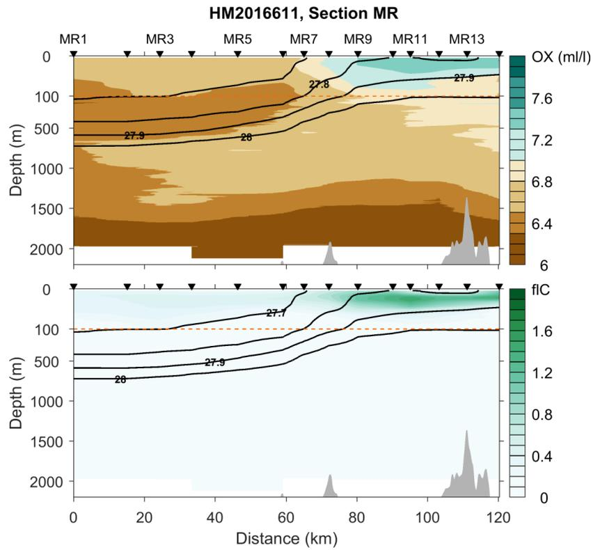
Figure 25. Contours of dissolved oxygen (OX) and fluorescence (fIC) for the MR section. Isolines of potential density anomaly ( $\sigma_\theta$ ) are also shown (black) on each panel. Note the change of vertical scale at 100 m.
