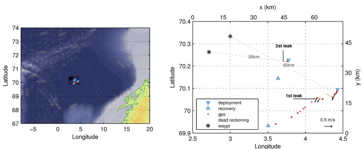
Figure 15. (left) Map showing the general location of deployment of Gnå. (right) enlarged view showing details of deployment and recovery, depth-averaged currents when available, way points, and the position when abort due to leak occurred.
