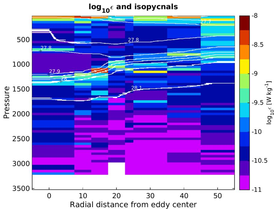
Figure 20. 50-m bin-averaged turbulent kinetic energy dissipation rate (logarithmic scale) across the eddy, measured by VMP5500 and VMP6000 pair. Averaged and pre-processed from shear 1 and 2 channels (bad segments and spikes were removed, further processing may be needed). The largest dissipation rates occur in the main deep thermocline/pycnocline.
