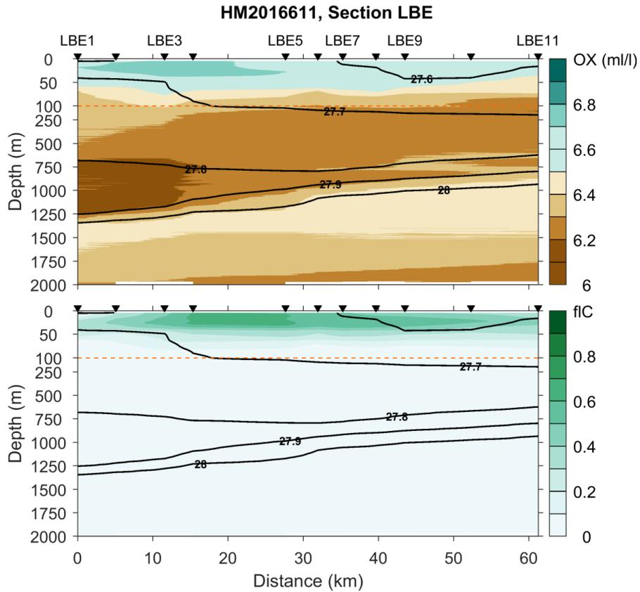
Figure 19. Contours of dissolved oxygen (OX) and fluorescence (fIC) for the LBE transect. Isolines of potential density anomaly ( $\sigma_\theta$ ) are also shown (black) on each panel. Distance is relative to the eddy center, which propagates in time. Note the change of vertical scale at 100 m.
