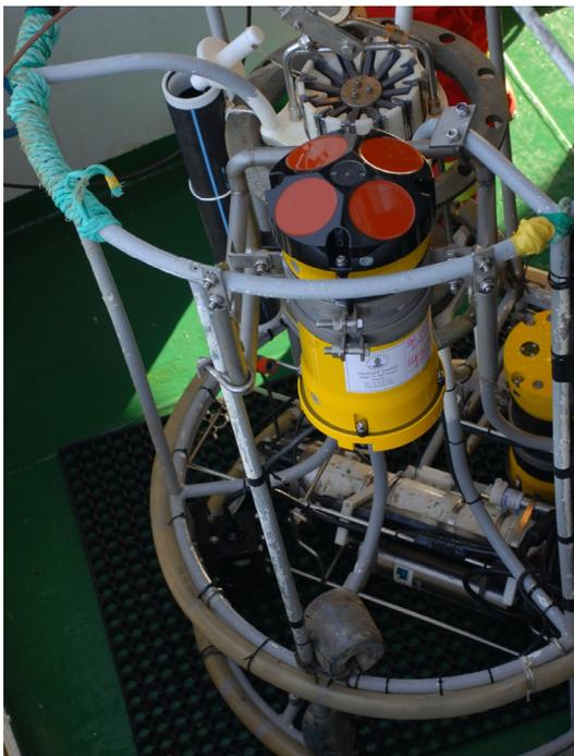
**Figure 6.** The CTD rosette together with the CTD sensors, one 5-liter Niskin bottle, a down and uplooker ADCP, and a benthos altimeter installed. The transducers of both ADCPs and the altimeter have a non-obstructed path. The position of the lead weights and the ADCPs are adjusted to have a negligible tilt of the entire system.
