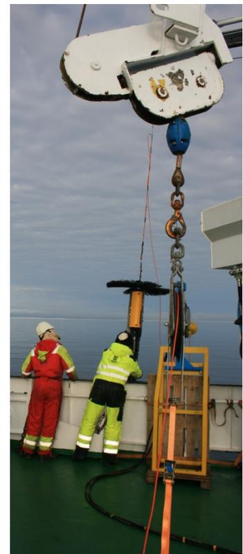
Figure 10. The set-up, on deck, of the VMP microstructure profiling system. The hydraulic winch (above); the cable is fed through a block supported by the crane in the middle. The block is fastened by straps to the deck to avoid swings due to wind and ship's roll. The tether then is fed into the line-puller (right) fastened to the ships' railing. In addition to the winch operator, a second person observes the cable in water during the deployment, and assists with deployment and recovery.
