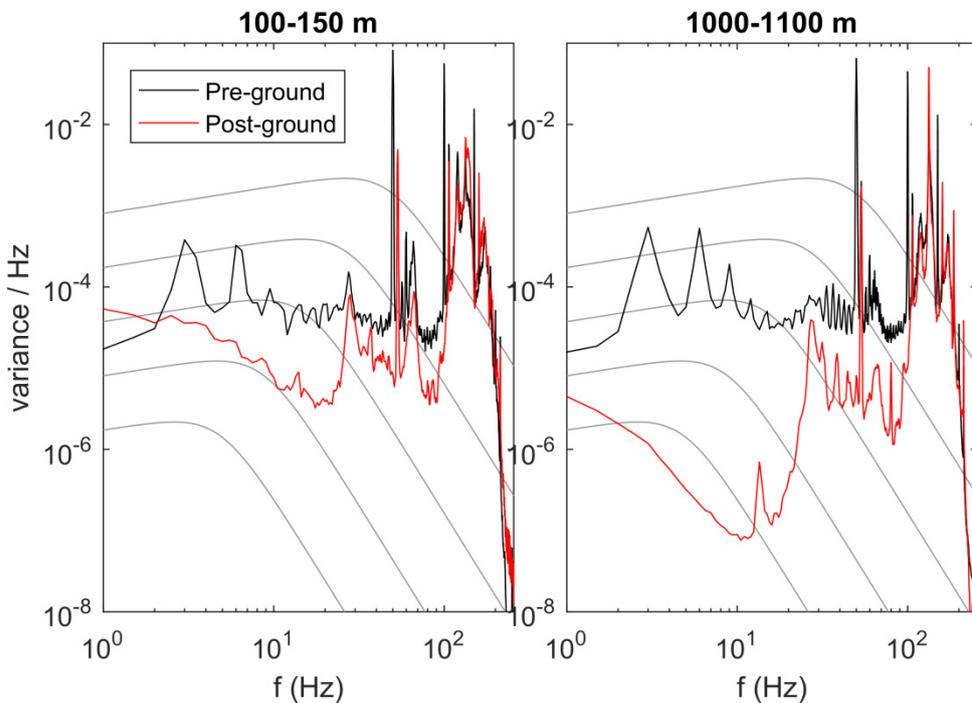
Figure 13. Shear spectra (probe 1) over two selected segments of 100-150 m and 1000-1100 m depth range using the data from cast 9 (before grounding) and cast 11 (after grounding). Spectra from other channels show a similar contamination but shear probes are the most affected.
