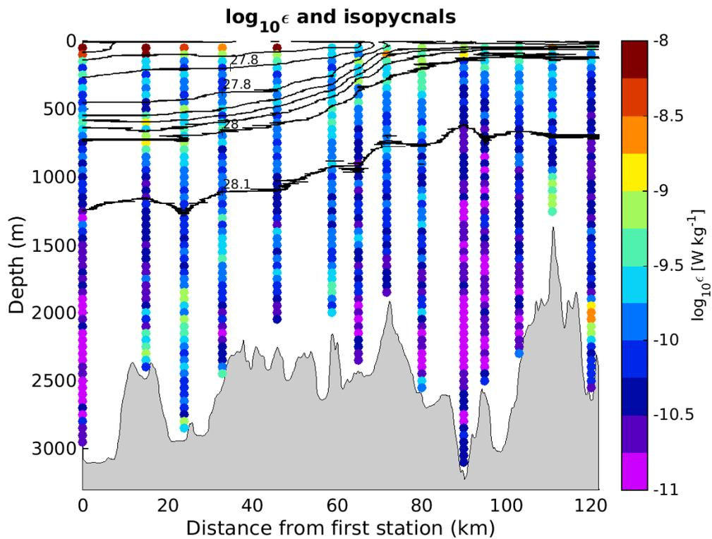
Figure 26. Dissipation rate profiles and contours of density along the MR section obtained using a series of VMP5500 and VMP6000 casts. Dissipation rate is from combined shear 1 and 2 channels. Bad segments and spikes were removed before passing through a 50-m bin-average.
