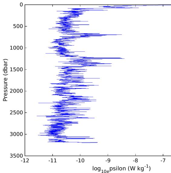
Figure 21. Dissipation rate profile at the eddy center. Two maxima were found at the location of the pycnolines: the shallowest at 700 m is in between the two homogeneous layers of the eddy, the deepest around 1300 m marks the upper boundary of the cold deep/bottom waters.
