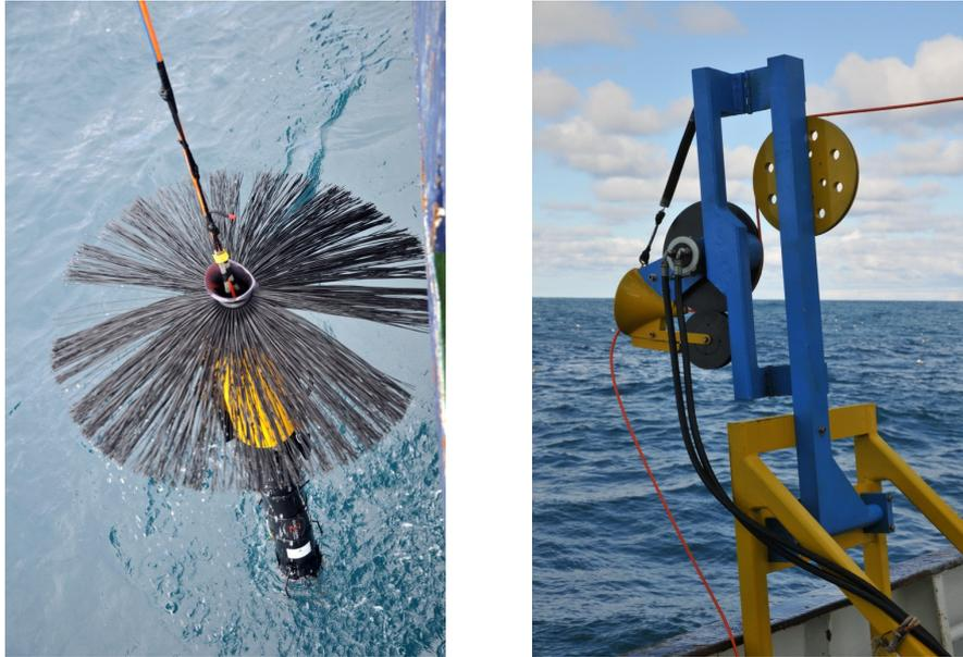
Figure 11. (Left) The VMP profiler during deployment. The brushes provide the drag for the profiler. Drag, together with the buoyancy elements (yellow) set the nominal sink velocity of the profiler. Note the recovery line attached to the cable which allows recovery by a crane without damaging the cable. (Right) The hydraulic line-puller.
