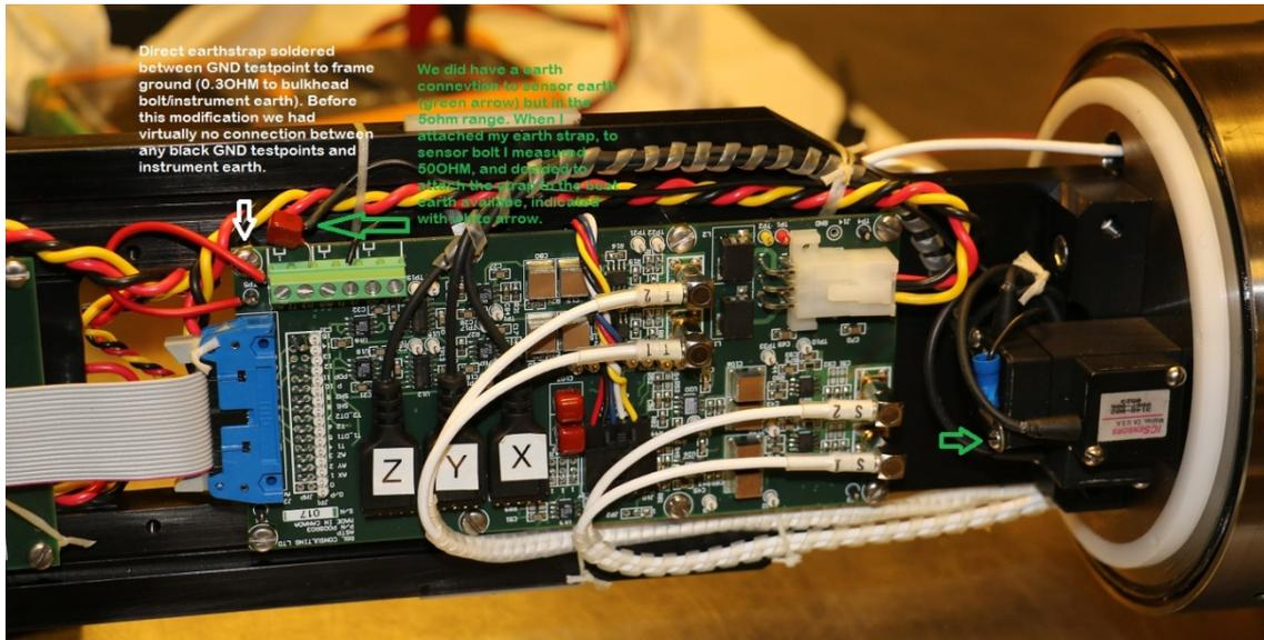
Figure 12. Grounding of the VMP2000. (Photo: Helge Bryhni)
