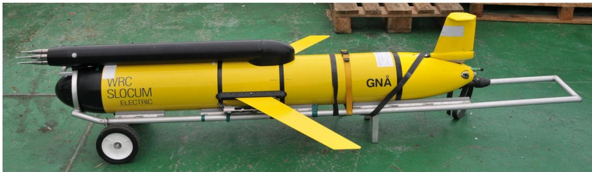
Figure 14. Photo of the glider Gnå mounted with MicroRider, strapped on the transportation trolley.
