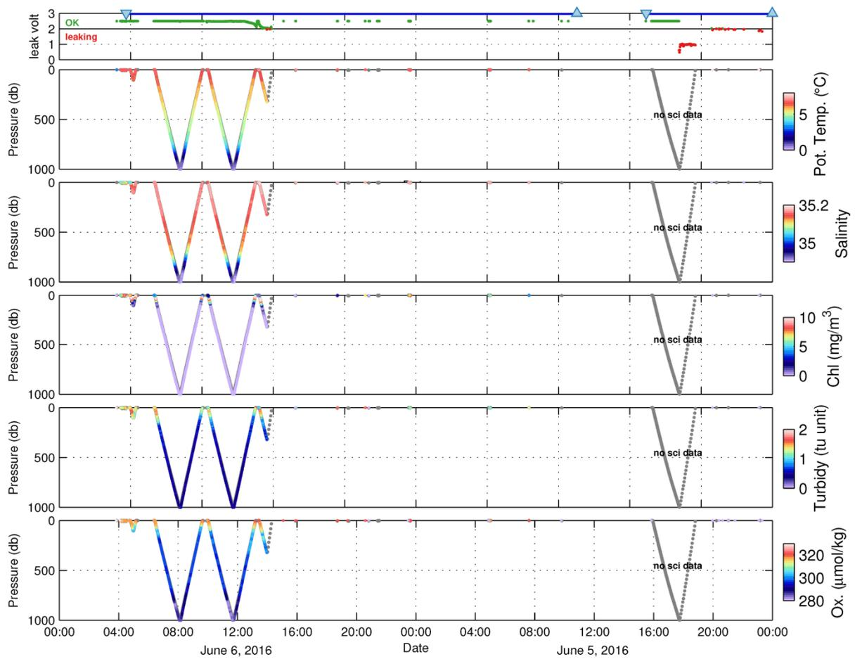
Figure 16. The upper panel shows the evolution of leak voltage throughout the deployments, with values indicative of a leakage marked in red. Lower panels: time-depth profiles color coded for science sensors. During the second deployment, no science data is available.
