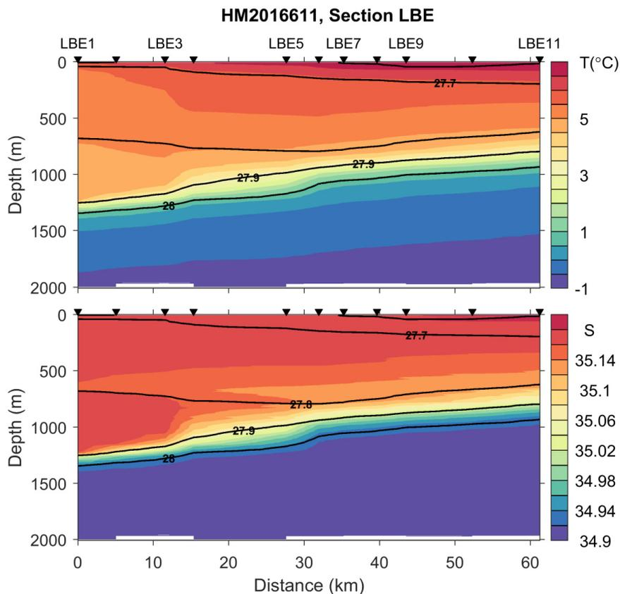
Figure 18. Contours of potential temperature ( $\theta$ ) and practical salinity ( $S$ ) for the LBE transect. Isolines of potential density anomaly ( $\sigma_\theta$ ) are also shown (black) on each panel. Distance is relative to the eddy center, which propagates in time. The center location is not accurately calculated for this presentation.
