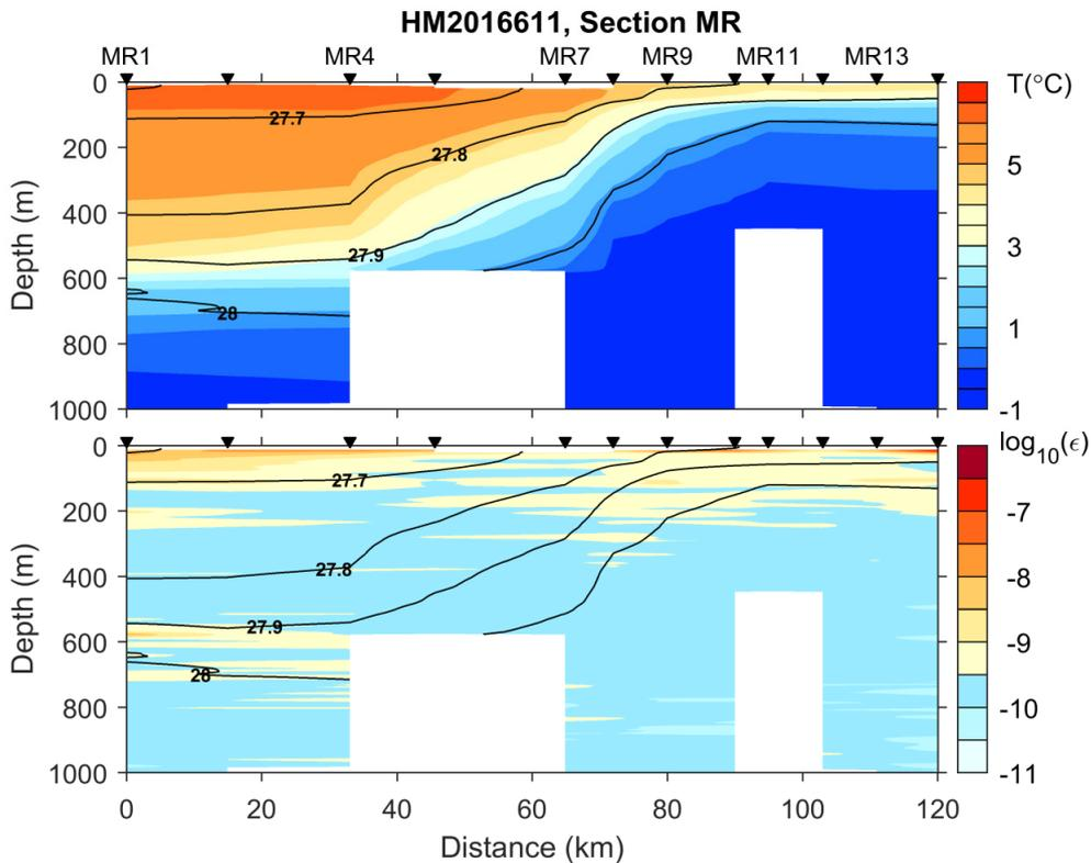
Figure 27. Temperature and dissipation rate contours measured by the VMP2000 in the upper 1000 m along the MR section. Isopycnals are drawn at 0.1 intervals.
