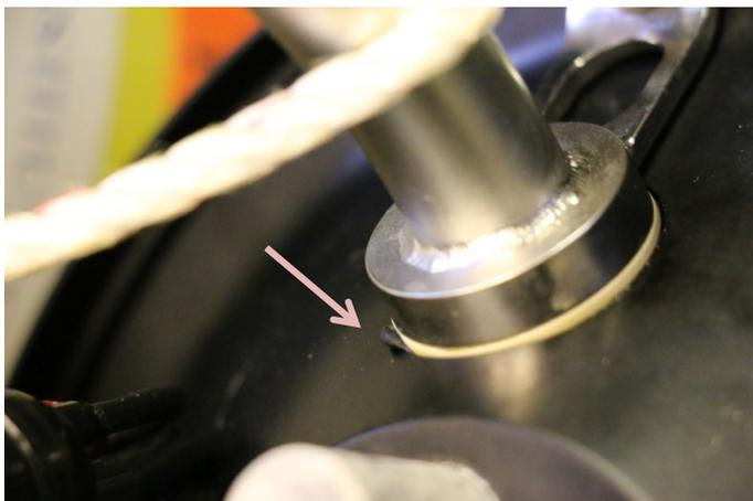
Figure 17. A zoom in to the aft section of Gnå where the tail fin is mounted on the pressure case. Note the damaged O-ring (arrow) that cause the leak. (Photo by H. Bryhni)
