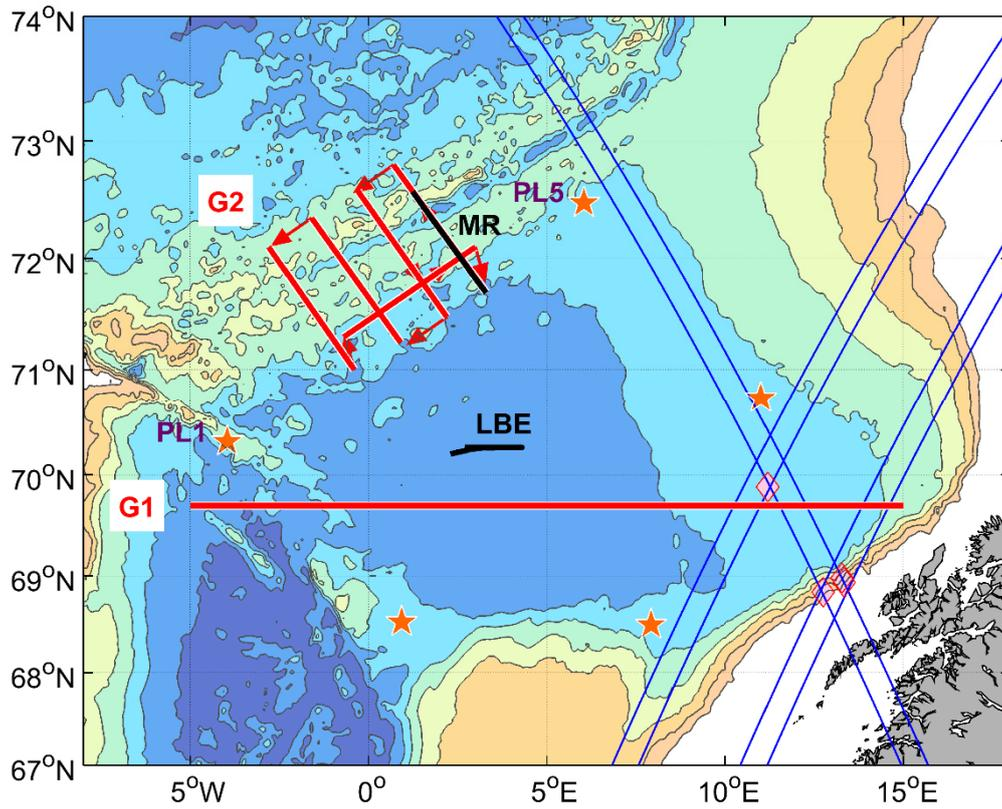
Figure 2. Station map, HM 2016611. G1 and G2 are the idealized mission tracks for Seagliders. Pentagrams mark the sound source moorings, PL1 to PL5 (counterclockwise). Oceanographic moorings are marked by diamonds (see Figure 3 for an enlarged map). Black traces (LBE and MR) mark the process study stations during the cruise. Relevant satellite (Altika) tracks are shown for reference (blue).
