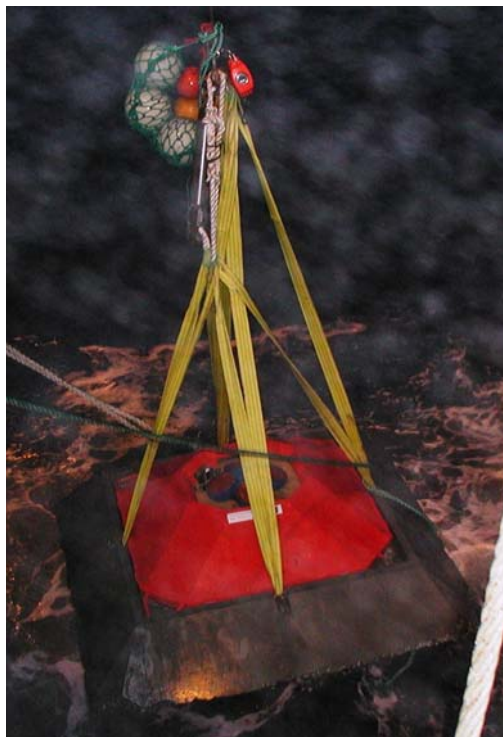
Figure 2. (left) The trawl-proof frame during deployment in summer 2003. (above) A close-up of the instruments before the 2006 deployment. The ADCP transducers are covered by the yellow protective cap removed before the deployment. The blue case on the left is the external battery unit. Horizontally installed is the Sea-Bird Microcat SBE37SM. (Pictures by F. Cleveland.)
